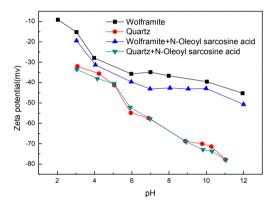
Fig. 5. Effect of N-oleoyl sarcosine acid on the zeta potential of wolframite and quartz
