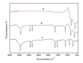
Fig. 6. Infrared spectrum in the absence and presence of N-oleoyl sarcosine acid (a – wolframite, b – wolframite after interacted with N-oleoyl sarcosine acid, c – N-oleoyl sarcosine acid)
